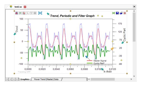
Here is the **blue curve** (the original trend) the original measurement data, connected with straight lines (polylines or when closed, this is called a polygon). These data points are fitted (filtered) with a 'Simple Moving Average' algorithm and gets the **red curve** (a fitted/filtered trend). Altogether, measurement data, polylines and red curve are belonging to one Graph, here the so-called Master Signal.
