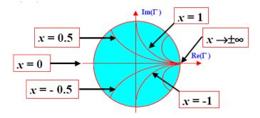
The Smith diagram can be used for line admittances, by shifting the space reference to the admittance location. After that, one can move on the chart just reading the numerical values as representing admittances. Let's review the impedance-admittance terminology:
