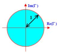
From a mathematical point of view, the Smith diagram is simply a representation of all possible complex impedances with respect to coordinates defined by the reflection coefficient.
