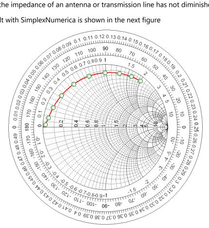
The Smith diagram is the result of the mapping of the right Gauss' number level into a circle area.
